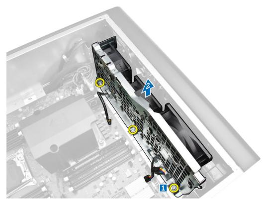
**10.** Insert the fan cable through the opening to release the system-fan module.
