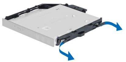
8. Lift the optical drive and remove it from the bracket.
