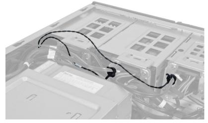
5. Open the latch securing the HDD thermal sensor and remove it from the computer.
