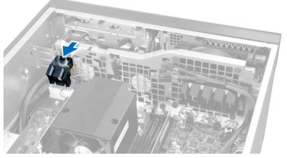
5. Lift the PCIe card retention in an upward direction to remove it from the computer.
