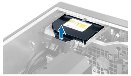
6. Slide the optical drive out of its compartment and lift it up to remove it from the computer.
