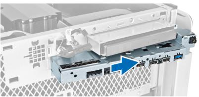
7. Remove the screws that secure the USB 3.0 module to the I/O panel assembly and remove it from the computer.
