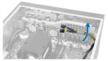
7. Route the system-fan cable through the opening in the system-fan module.
