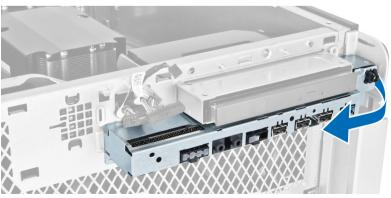
6. Slide the opposite edge of the I/O panel assembly outward to disengage the I/O assembly from the chassis.
