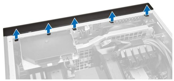
**4.** Rotate and pull the bezel panel away from the computer to release the hooks on the opposite edge of the bezel from the chassis.
