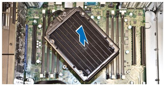
6. Remove the screws that secure the heatsink bracket and remove the bracket away from the system board.
