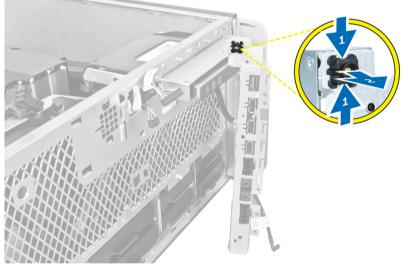
4. Remove the power switch from the computer.
