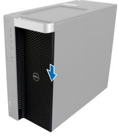
**3.** Keep the latch pushed down, and pull the front cover in an outward direction to remove it from the computer.
