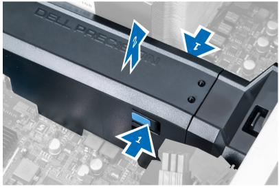
**4.** Press down on the release latch on the other side of the memory shroud module to release it from the chassis.
