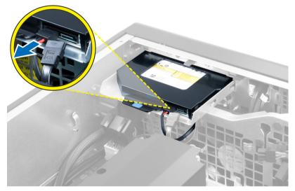
5. Pull up the blue release tab to release the latches that secure the optical drive.
