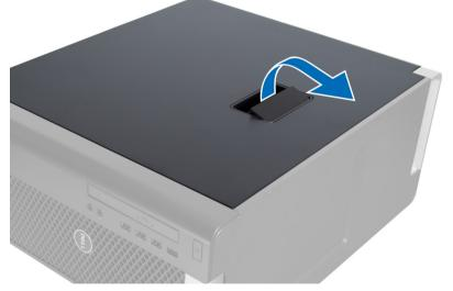
3. Lift the cover upward to a 45-degree angle and remove it from the computer.
