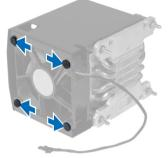
4. Remove the heatsink fan from the heatsink assembly.
