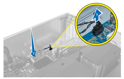
4. Unroute the HDD thermal-sensor cable from its securing clips on the chassis.
