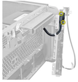
8. Remove the screws that secure the I/O panel and remove it from the I/O panel assembly.
