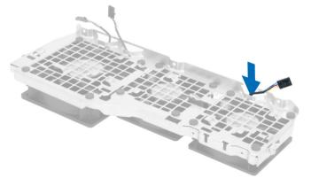
**11.** Remove the grommets that secure the system fan , lift up the fan and remove it from the fan assembly.
