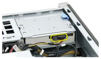
4. Press the release latch and slide the optical drive outward to release it from the drive bay [1, 2].
