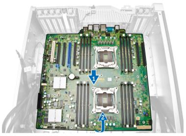
6. Lift the system board in an upward direction and remove it from the computer.
