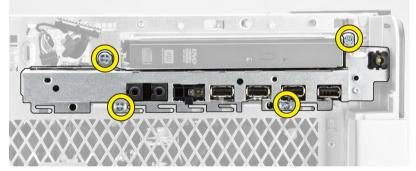
5. Pull the I/O panel assembly in a direction opposite to the computer to release its edge from the chassis clip.
