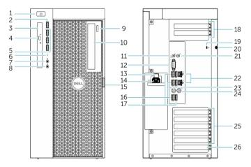
Figure 1. Front and Back View of T7910 Computer
