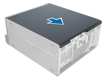
**4.** Lift the right cover at a 45–degree and remove it from the computer.
