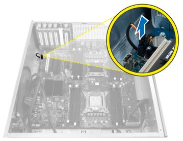
4. Route the cable from below the computer chassis as indicated.
