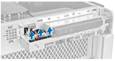
4. Remove the screws that secure the I/O panel assembly to the computer chassis.
